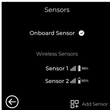
3. Pair the sensor with the Nuve thermostat. The system prompts you to remove the battery tab from the sensor or press and hold the reset button for two seconds.
