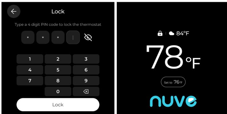
To unlock the thermostat, tap the screen and enter the 4-digit PIN code. If you enter the wrong PIN code, you have two additional attempts. After three incorrect entries, PIN input will be disabled for 2 minutes. You can also unlock your device from the Mobile app (Menu - Unlock.)
