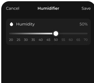
3. In the dehumidifier page, move the slider to set the humidity percentage above which to dehumidify the air. When you are done, click Save.
